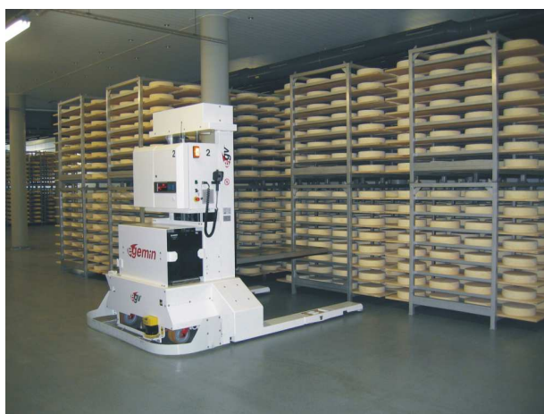
Figure 5.1: An AGV at work in a cheese factory
